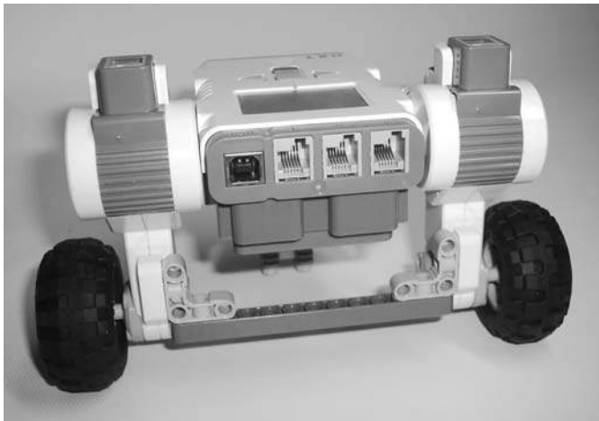
Figure 10-3: The robot in Figure 10-2 after being braced with beams connecting the motors
