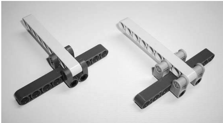
Figure 10-6: Two examples of strong brace connections
