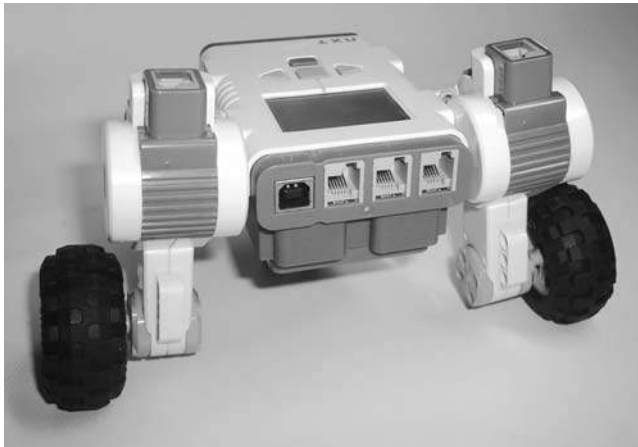
Figure 10-2: A robot that hasn't been braced can have a weak structure.
