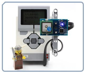
**FIGURE 3:** Attach the dGPS to the EV3 Intelligent Brick with an open center frame liftarm.
