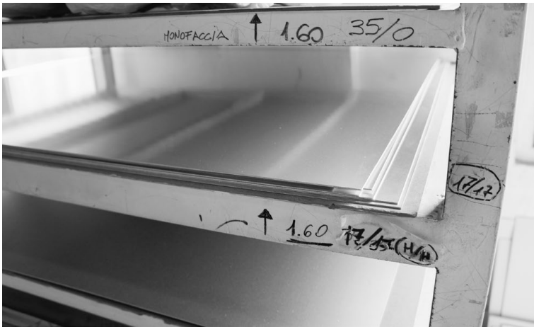
A stack of copper sheets waiting to become Arduino boards
