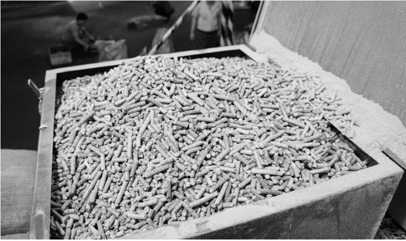
Compressed sawdust pellets, used to fuel the ingot smelter
