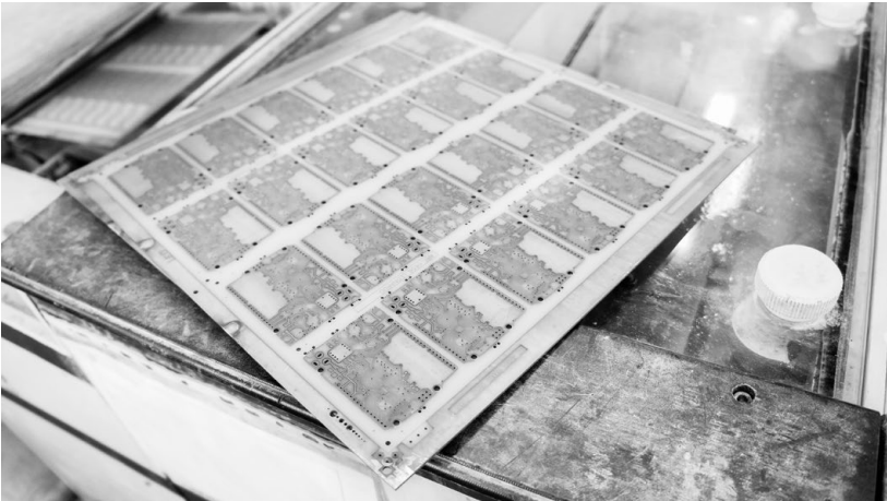
A panel etched of unwanted copper
