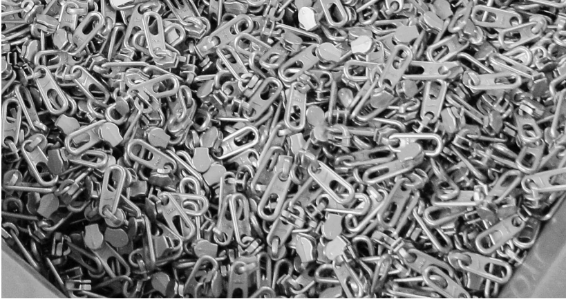
Finished zipper puller and slider assemblies
