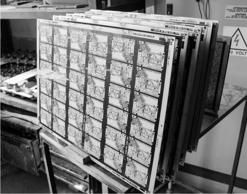
Panels of Arduino Leonardo boards after going through a series of chemical baths
