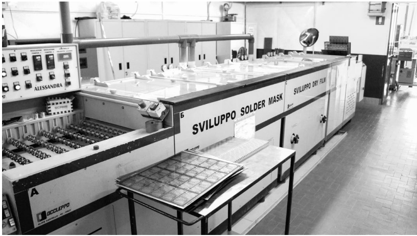
The machine that develops the photoresist
