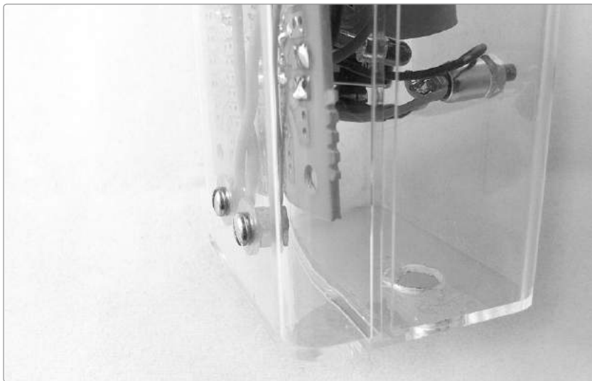
FIGURE 6-18: Note the opposing orientations of the body contacts (the two screws on the left face of the case) and the power switch (on the right face). You can also see the larger hole at the end of the case, which is for the talk tube.
