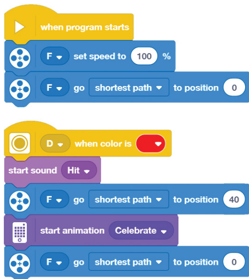
Figure 2-5: The complete program for the Baseball Batter uses the color sensor to detect the ball.
