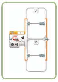
Figure 6-1: The Switch block
