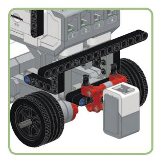
Figure 6-3: Color Sensor position for following a line
